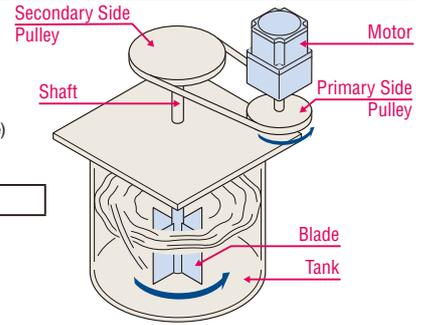
Specifications of the Tank and the Agitated Object
